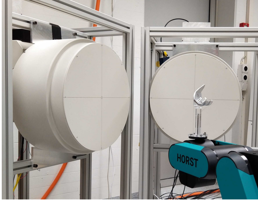
Fig. 1: Schematic of the dual-plane X-ray imaging setup.
