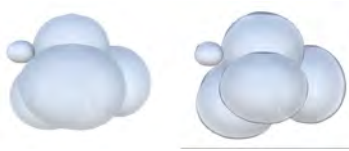
Fig. 3. Comparison of perspective (left) and orthographic (right) camera projections when used to view 3D reconstructions.
